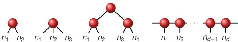
Figure: Different examples for TTN's (from left to right): matrix, Tucker tensor, binary TTN, matrix product state.
